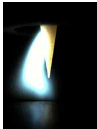
Low-quality tungsten: typically sideways arc ignition, the arc flashes and wanders slowly to the electrode tip which has to be cut off and reground.
