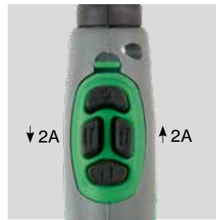
Up/Down module with 4-function key for adjustment of welding current incl. TIG-A-Tack function. The welding current is increased / reduced with 2 amps. Long press for constant increase / decrease. Art. no. ....80300063 * Applies to software versions as of 2.17
