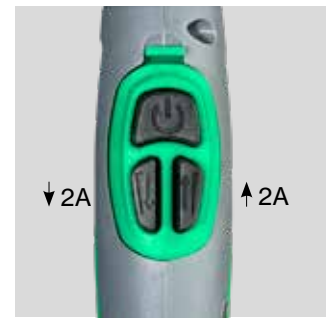
Up/Down module with 3-function key for adjustment of welding current. The welding current is increased / reduced with 2 amps. Long press for constant increase / decrease. Art. no. ....80300064* * Applies to software versions as of 2.17
